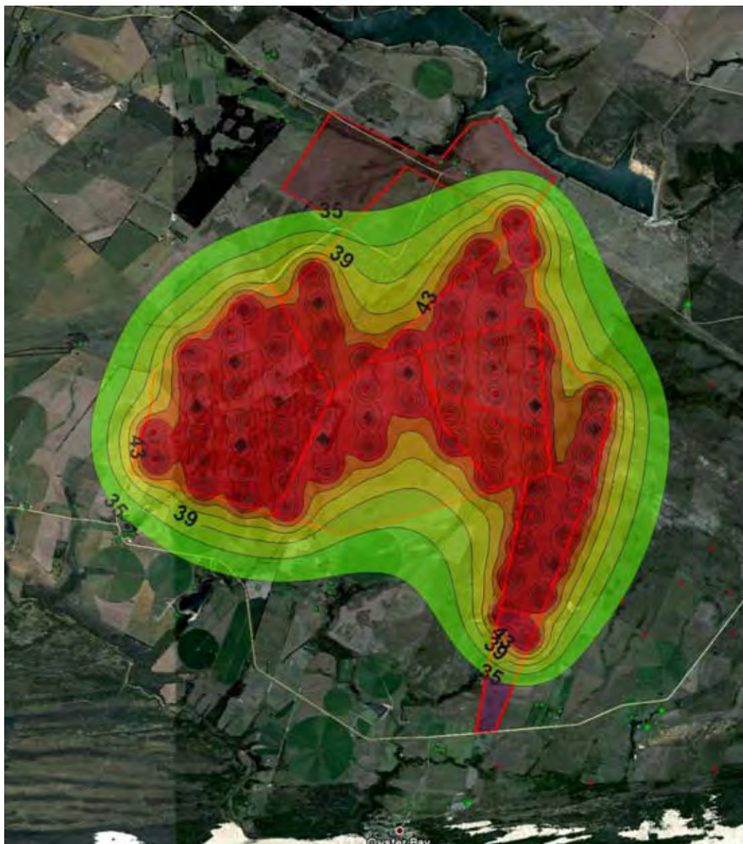
Figure 7.18: Projected Noise Levels (ISO model) from Oyster Bay wind turbines; Contours of constant sound levels for a 5 m/s wind (WTGs marked as red dots, PSRs as green dots)
