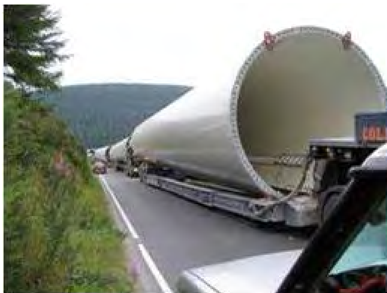
Figure 3.8: Typical abnormal load for transportation of wind turbine components in segments
