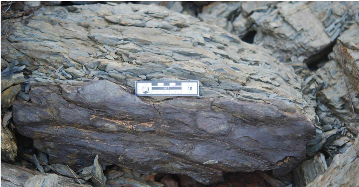
Figure 27: Mudstones of the Karies Formation exposed in a borrowpit at point 20 (Fig.1). water ripple marks are evident on surface facing viewer.
