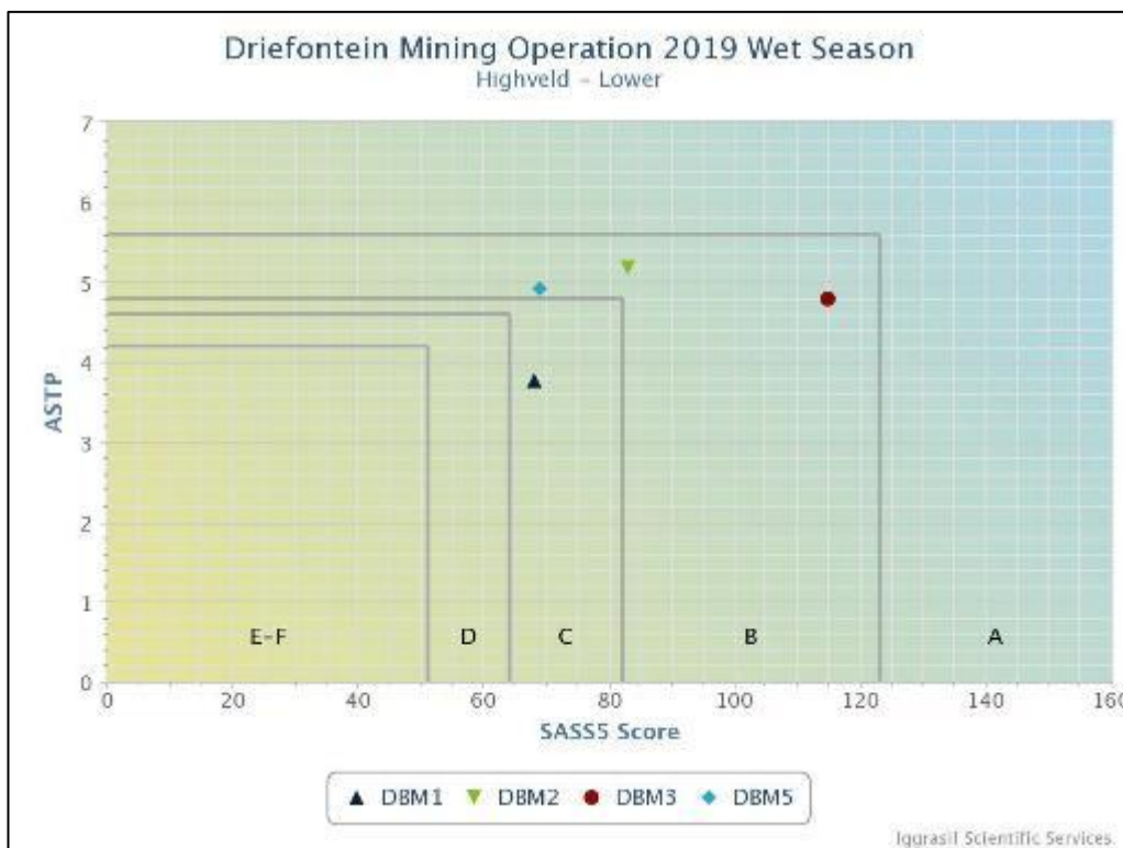
Figure 33: SASS5 Score and ASPT Plot for sampling points at Driefontein Mine in comparison to the biological bands for the Highveld Ecoregion (Lower zone) (Dallas 2007)
