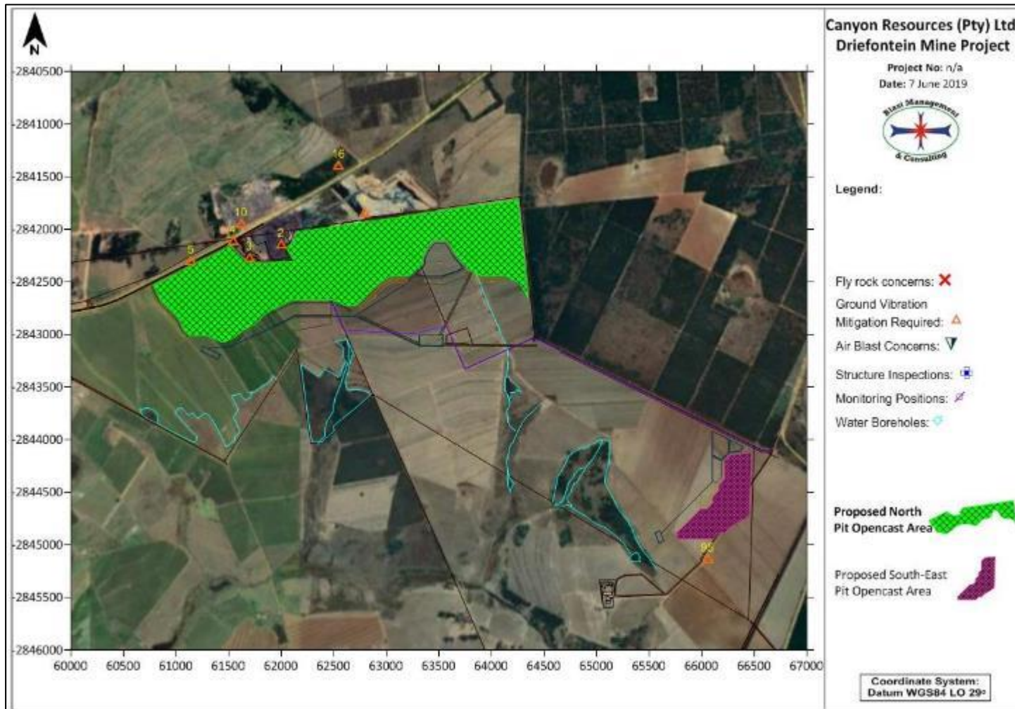
Figure 105: Structures identified at the pit areas where ground vibration mitigation will be required
