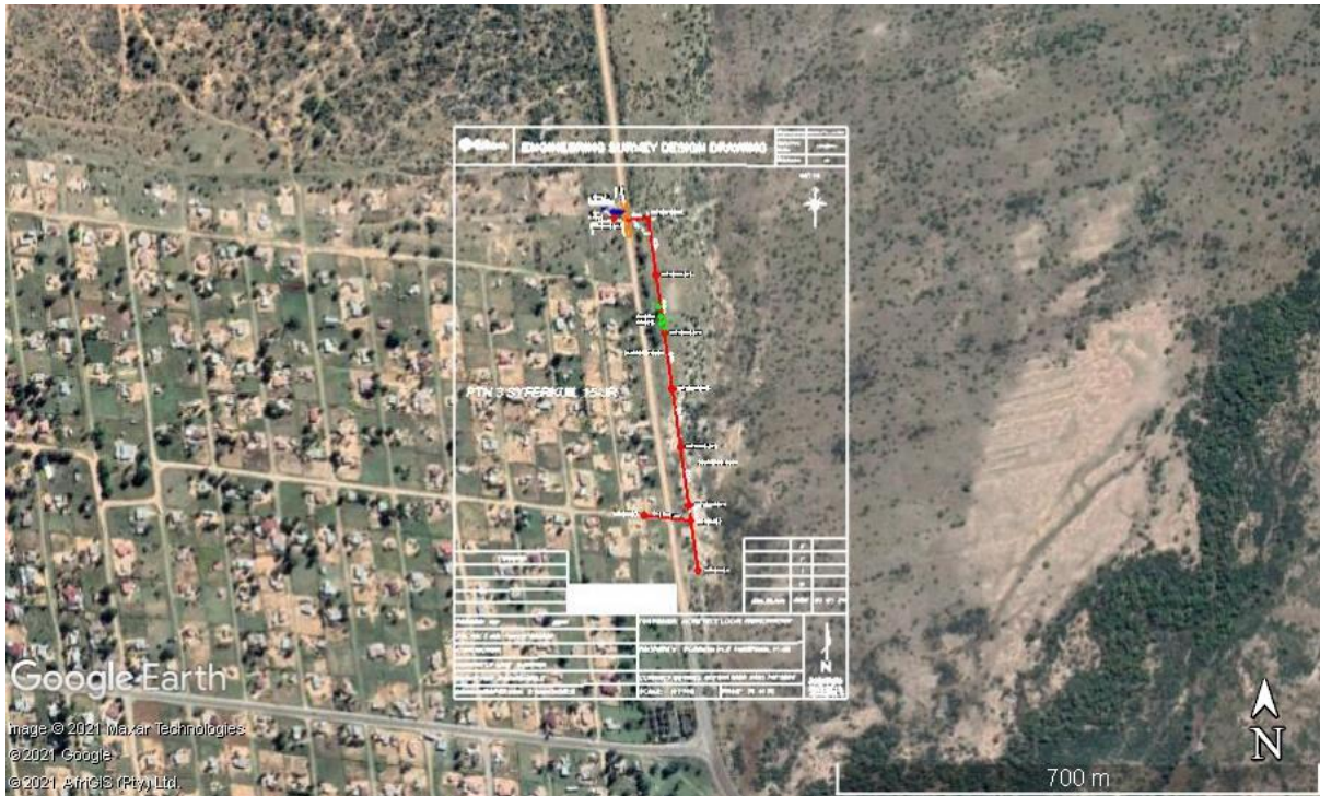
Figure 1: Google Earth map of the proposed construction of a 388.40m MV powerline from the existing line alongside the road, to a borehole pump for the Mogohlwaneng village on Portion 3 Syferkuil 15-JR in Moretele Local Municipality. Map supplied by TAP.
