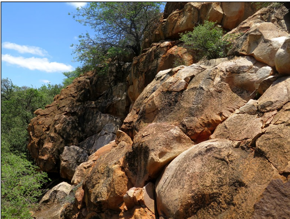
Figure 19. Massive, well-jointed and indurated Clarens sandstone in the Site 2 study area (N-facing scarp) showing rounded, conchoidal fracture in the foreground and scabby karstic weathering surface in the background.
