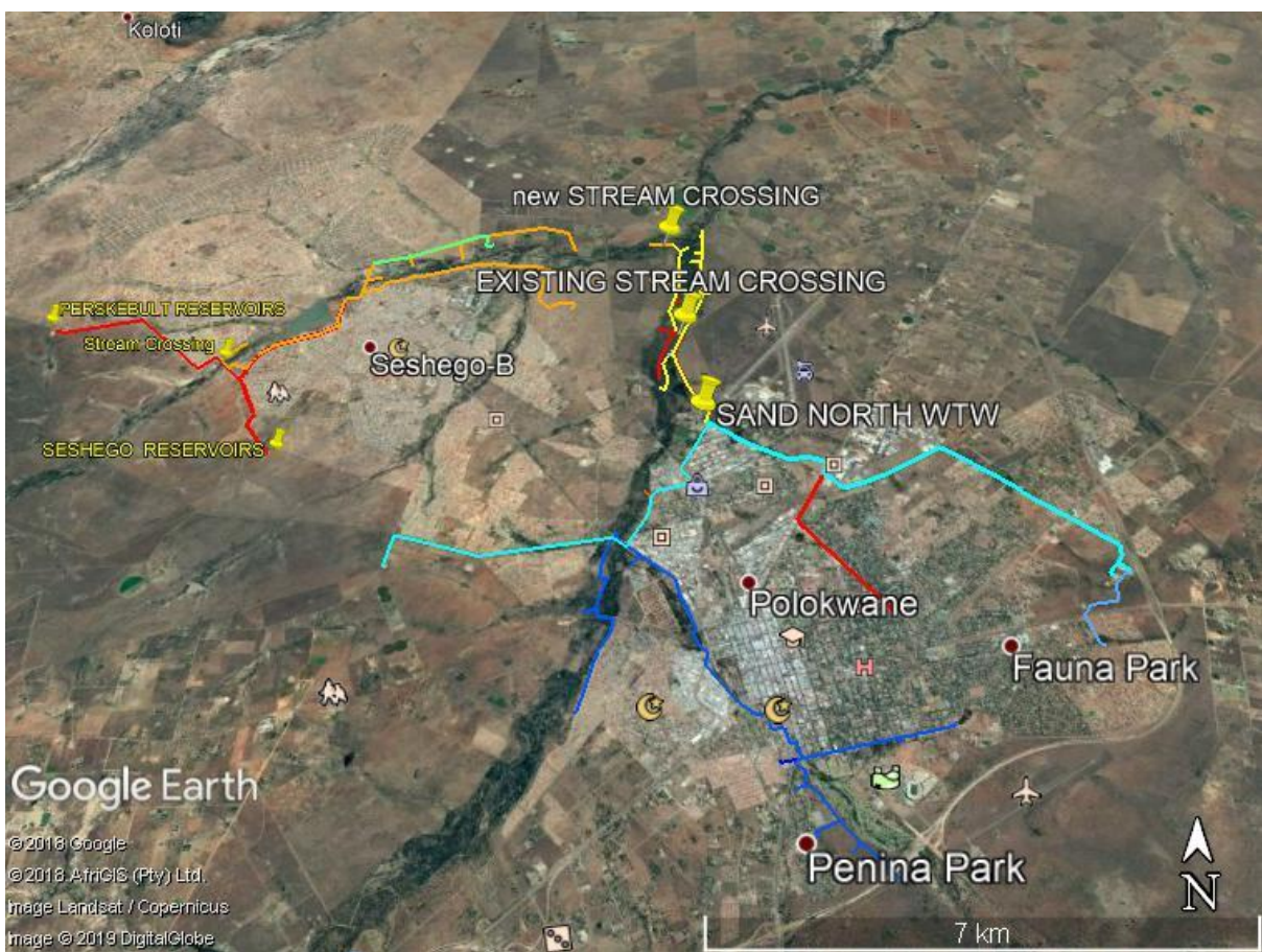
Figure 1: Composite Google Earth map showing the proposed routes of the pipelines around Polokwane, Limpopo Province. Three phase have been planned: Phase 1 - light blue and dark blue lines; Phase 2 - red, orange and green lines; Phase 3 - red and yellow lines. Map supplied by HCAC.
