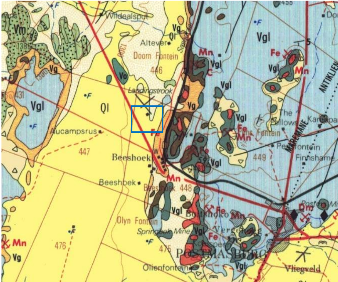
Figure 2: Geological map of the area around Beeshoek and Postmasburg. The location of the proposed project is indicated with the blue rectangle. Abbreviations of the rock types are explained in Table 2. Map enlarged from the Geological Survey 1:250 000 map 2822 Postmasburg.
