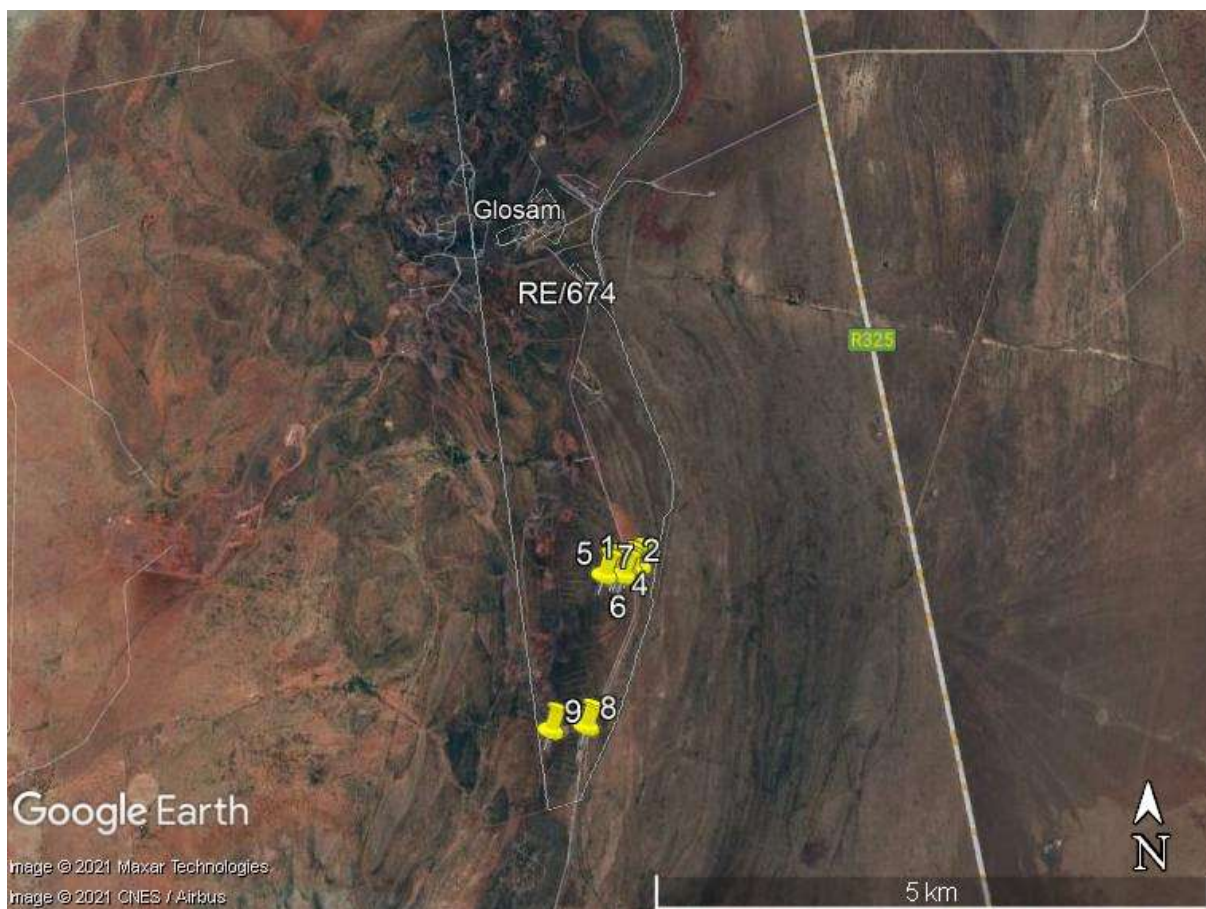
Figure 5: Google Earth map with GPS points and sites as indicated. Refer to Table 3 for site observations and related photographs (Figures 8-12). Stop 1 is the base of the test strip, moving uphill (westwards from Ghaap Plateau rocks to Kuruman Fm rocks). Strips are 5m wide and traverse from the valley to the ridge top (next property). Test trenches are at random positions within the test strip and are less than 1m wide and up to 2m deep.
