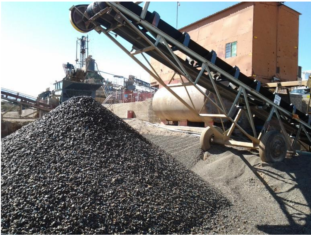
Figure 3: Thunderflex Dense Media Separation (DMS) Plant with Ferrosilicon recycling tank in the background and plant waste rock pile in the forefront.
