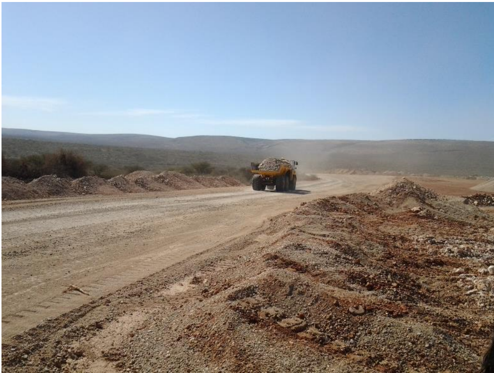
Figure 5: Screen reject being hauled to prospecting trenches as backfill.
