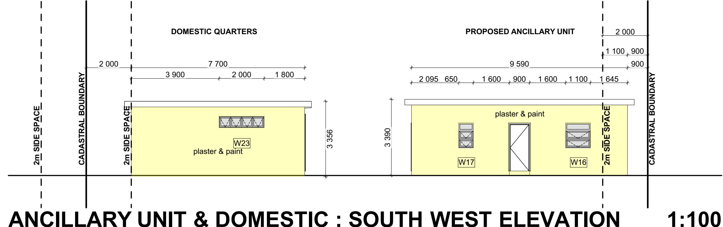
ANCILLARY UNIT & DOMESTIC : SOUTH WEST ELEVATION 1:100
