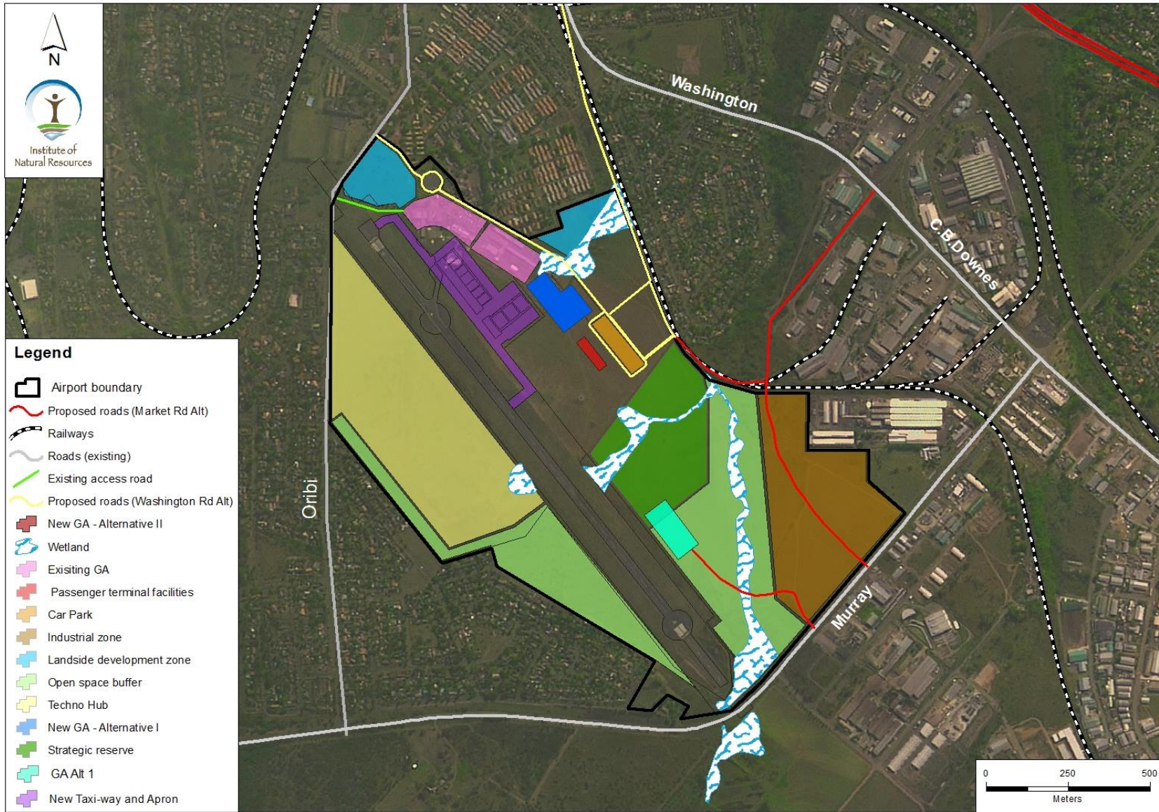
Figure 9: Layout and extent of the elements comprising of the phase 1 of the project
