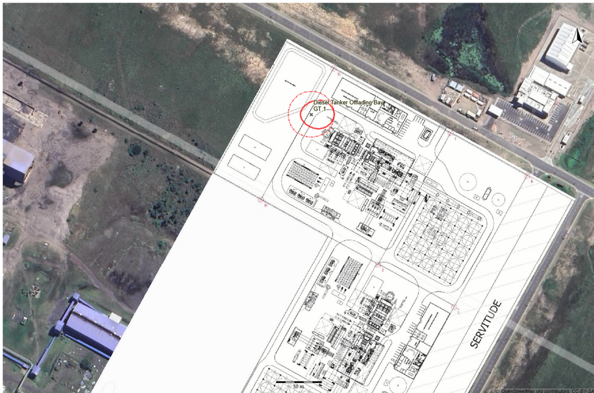
Figure 5-6: Thermal radiation from large diesel pool fires at the road offloading area at the assumed position at the Northern gas turbine area
