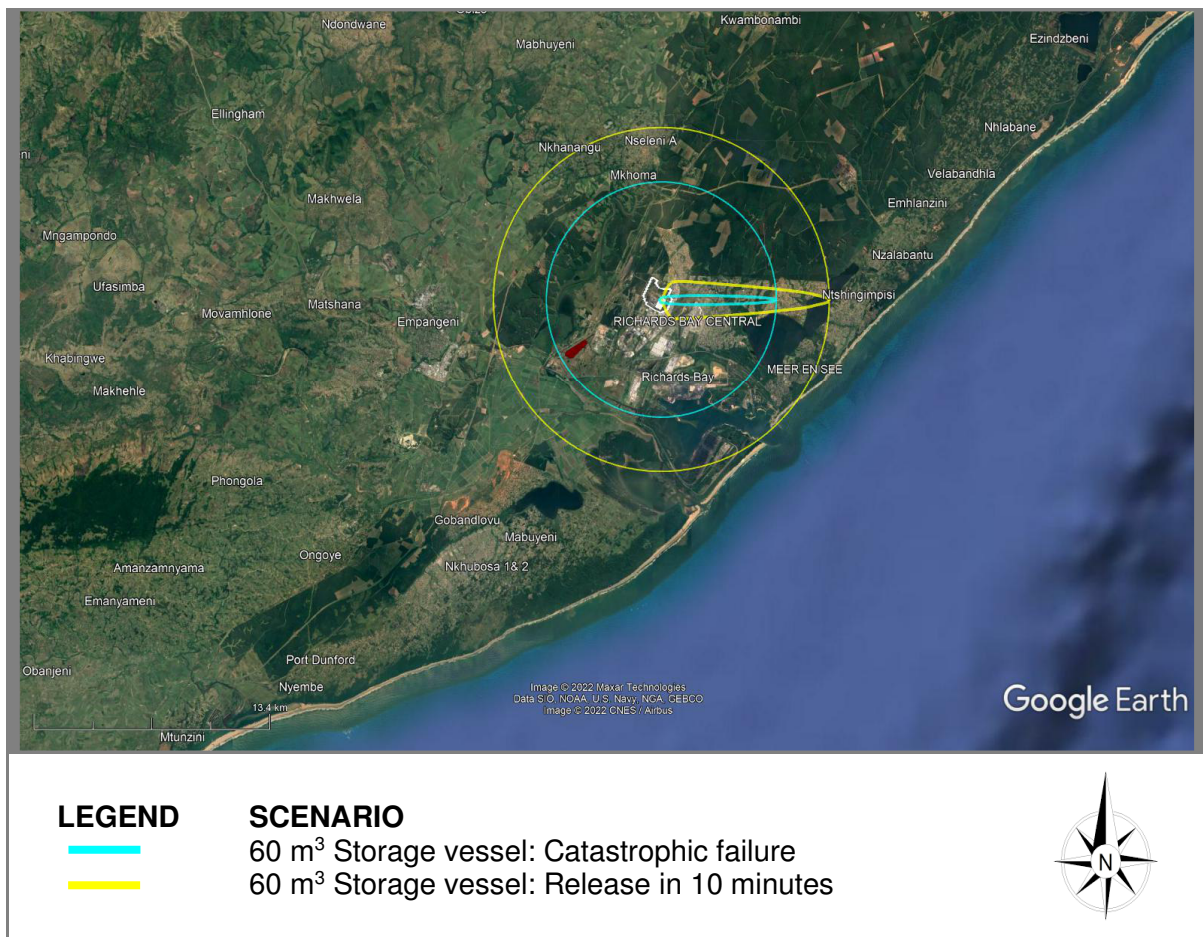
Figure 5-3: The extent of the ERPG-2 values of ammonia following a large release
