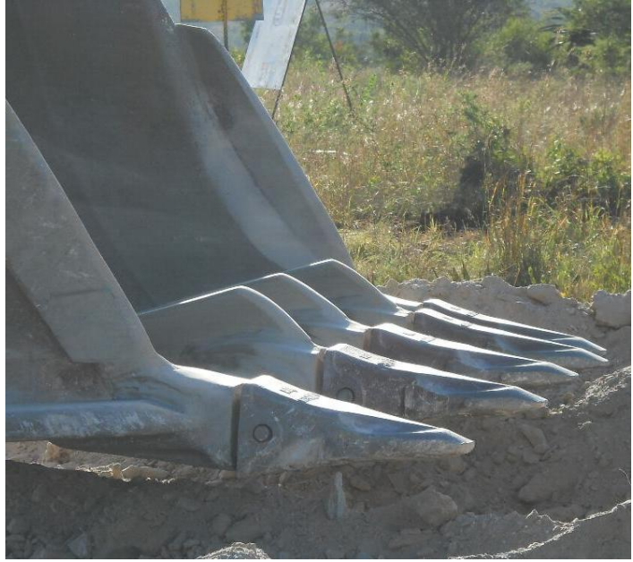
Fig 11. Clearly visible in the image at left are the bucket teeth before replacement the next day (at right).
