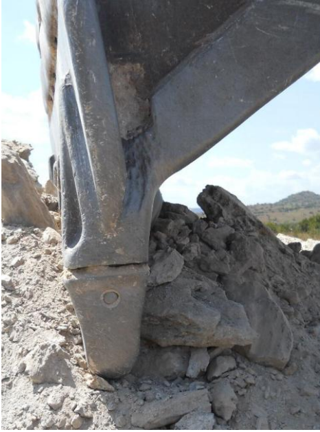
Fig 11. Clearly visible in the image at left are the bucket teeth before replacement the next day (at right).
