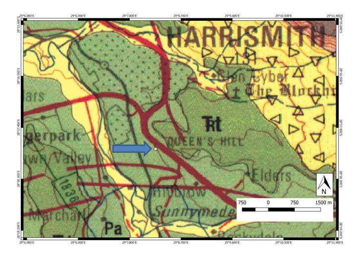
Figure 4: Extract of the 1:250 000 2828 Harrismith Geological map (Council of Geoscience) of the proposed Harrismith emulsion plant establishment, Free State. The proposed development is coloured in white and indicated by the blue arrow. The proposed development is located within the Late Permian sedimentary rocks of the Normandien Formation, Adelaide Subgroup (Beaufort Group of the Karoo Supergroup). Map drawn by QGIS 2.18.28.
