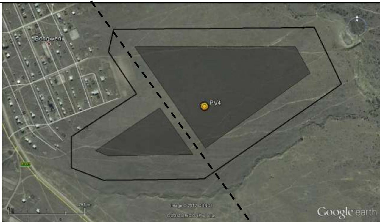
Plate 4.7 An aerial photo shows the surrounding degraded grassland with Bongweni bordering on the west. The shaded polygons represent the solar panel's footprint. The dashed line represents the existing power line layout.
