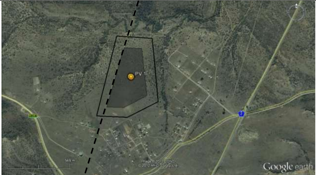
Plate 4.2. An aerial photo shows denser tree vegetation in the surrounding drainage systems. The shaded polygons represent the solar panel's footprint. The dashed line represents the existing power line layout.
