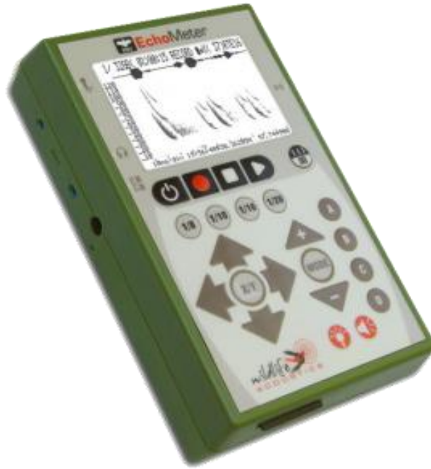
Figure 7-4 The EM3 detector used for manual bat activity surveys
