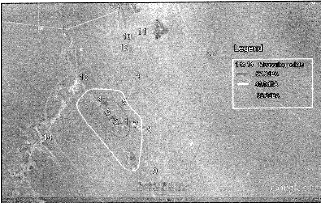
Figure 5: Noise contours during open cast activities at the proposed open cast mine.
