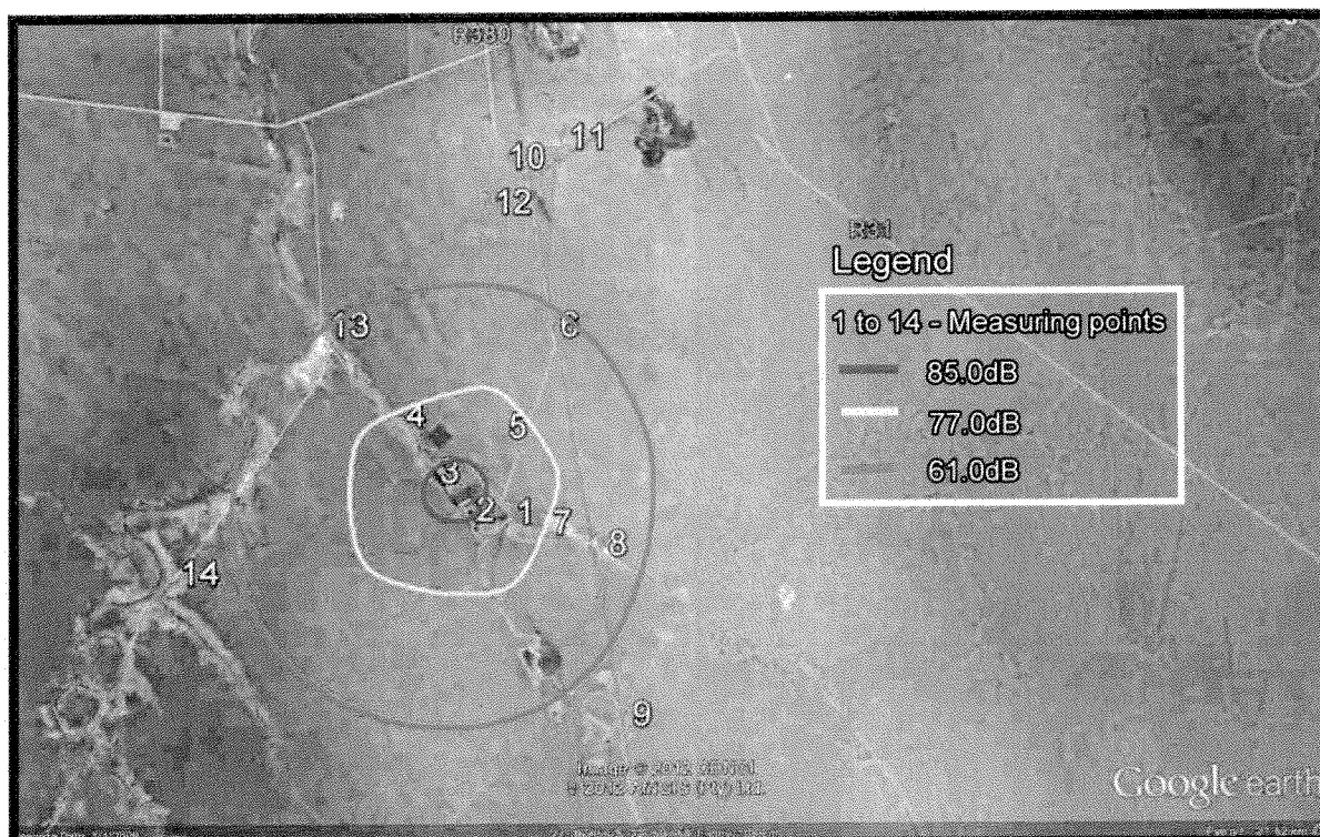
Figure 50 Air blast noise contour at the open cast pit.
