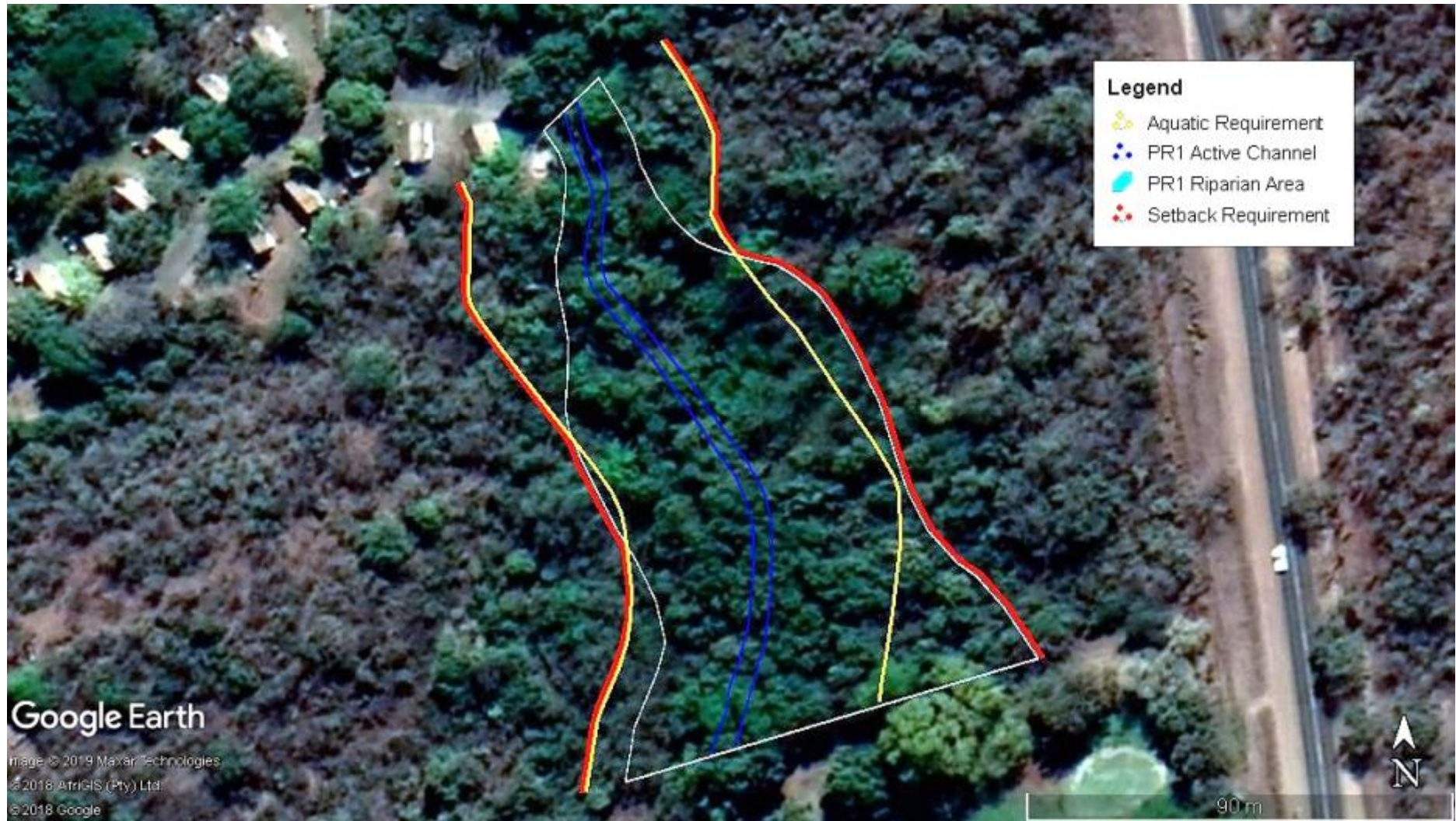
Figure 5-26: Delineation of the PR1-Riparian site's active channel edge, aquatic requirement, riparian edge and then the final setback requirement
