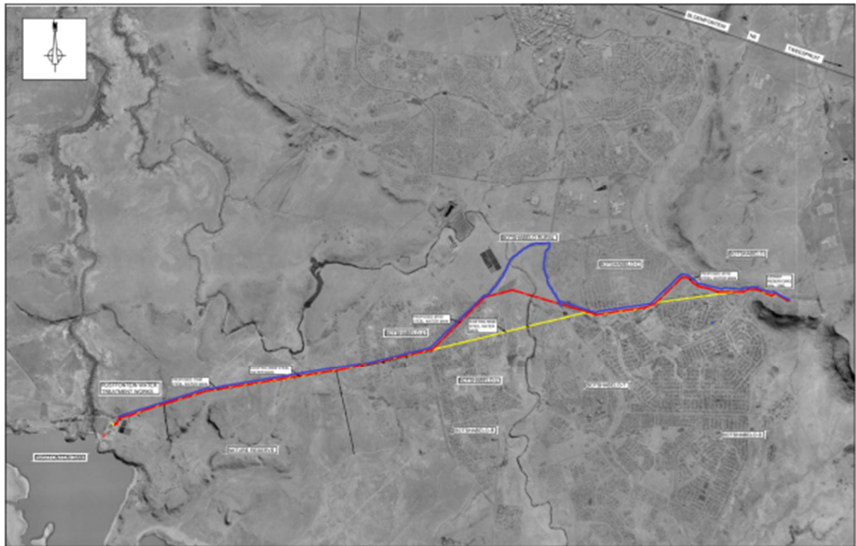
Figure 2.1 Site plan of existing (yellow) and the two alternative routes (alternative 1 – red; alternative 2 – blue) of the Bloemwater: RustfonteinDam/Botshabelo Water Supply Pipeline
