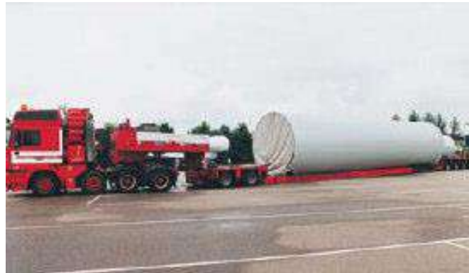
Figure 2.9: Tower section being transported.
