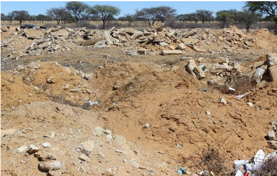
Plate 1.2: An example of inert waste (construction rubble) that is currently dumped at Piet Plessis
