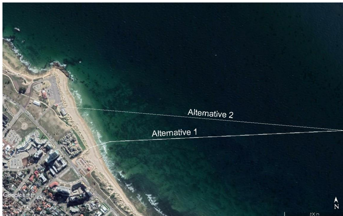
Figure 2: GoogleEarth image showing the routing of the proposed 2AFRICA/GERA (East) Cable System in shallow waters and the shore crossing alternatives at Pollok Beach, Summerstrand in Port Elizabeth.
