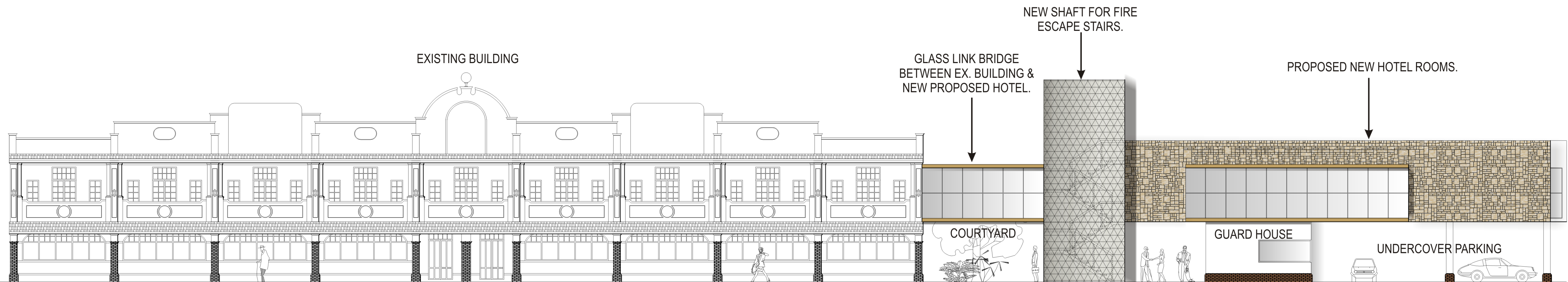
North Elevation (street frontage)
