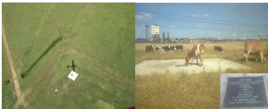
Figure 5.14.3.3(a): Typical Closed and Rehabilitated Vertical Shaft
