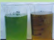
Vetiver grass will remove phosphate and nitrate from polluted water. The beaker on the left is before treatment; on the right 4 days later 90% P and 94% N removed
