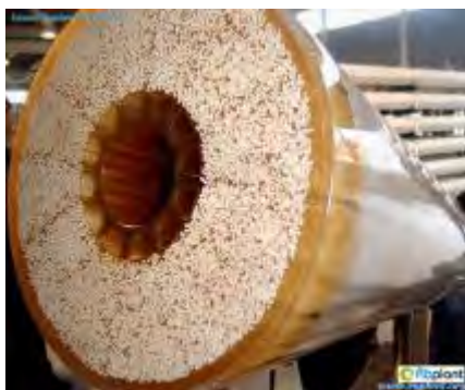
Figure 3.1.5.17.4 (c): Capillary UF Membrane Module and Typical UF Plant
