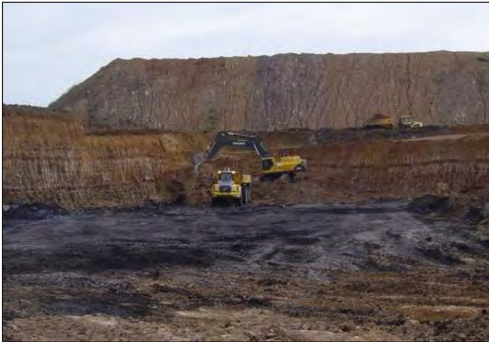
Figure 3.1.7.5 (a): Removal of Hard Overburden directly above Coal Seam
