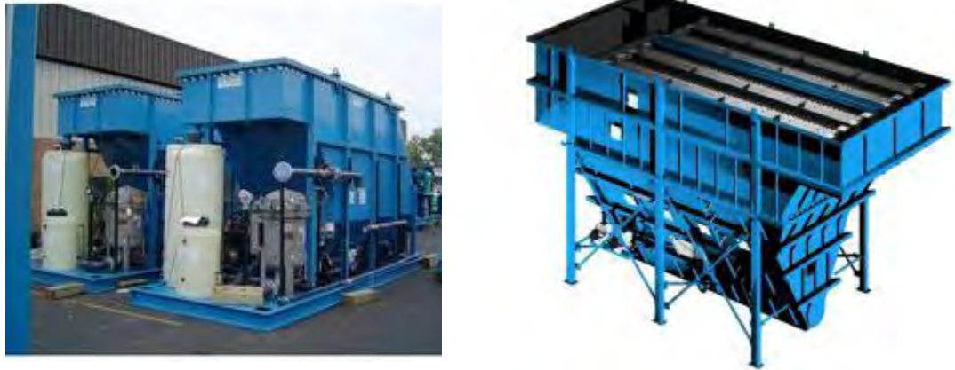
Figure 3.1.5.17.4 (a): Lamella Clarifiers
