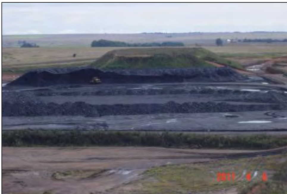
Figure 3.1.5.5 (a): Typical ROM Stockpile – note the sequential operation as well as the water management berms.
