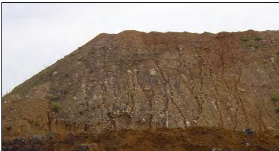
Figure 3.1.5.6 (a): Typical Overburden Stockpile – note the low carbonaceous content.
