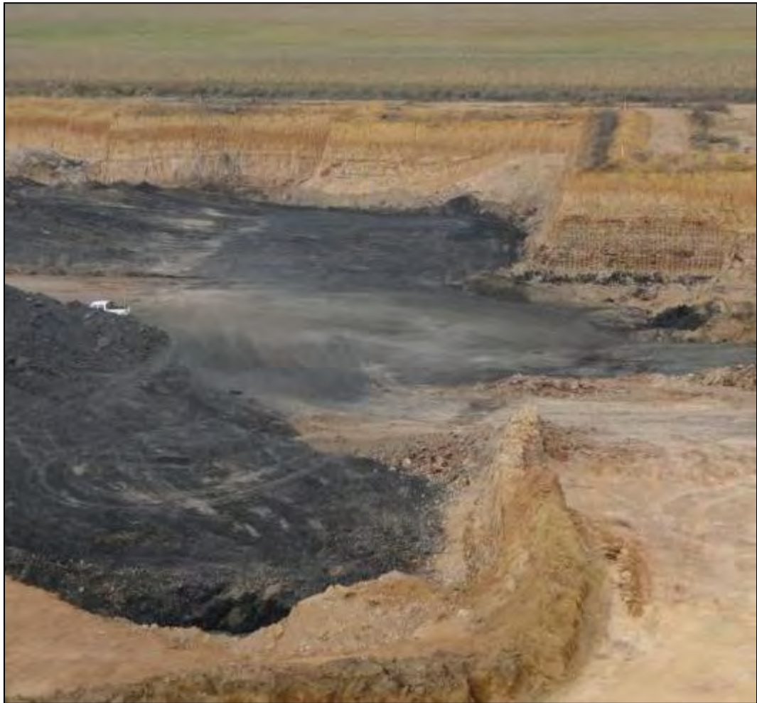
Figure 3.1.7.5 (c): Block almost ready to be Drilled, Blasted and Stripped of Coal
