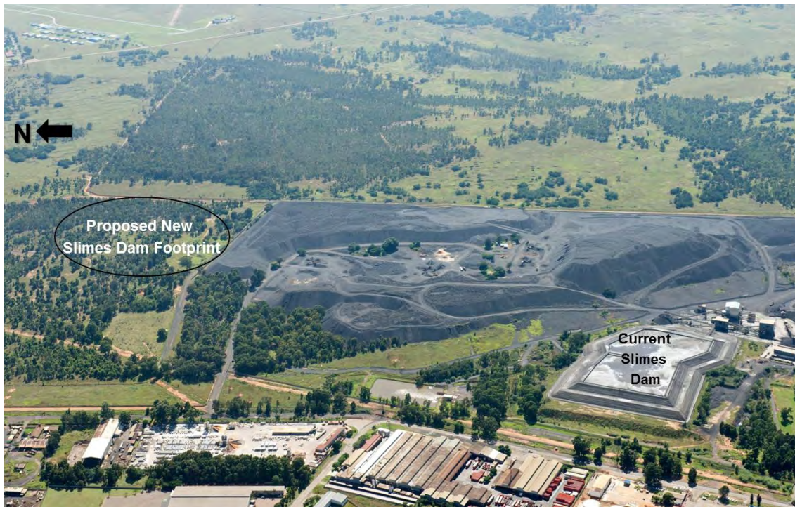
Figure 3.9.2(C): Best Alternative footprint (new Slimes Dam) and Existing Slimes Dam Footprint.
