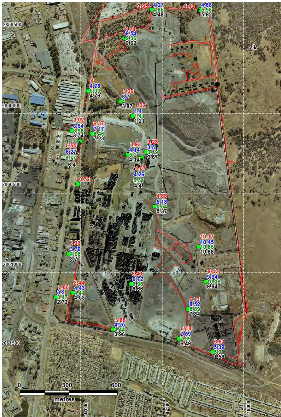
Figure 4.6(e): Ground water level data for 2012 – FSD monitoring boreholes.
