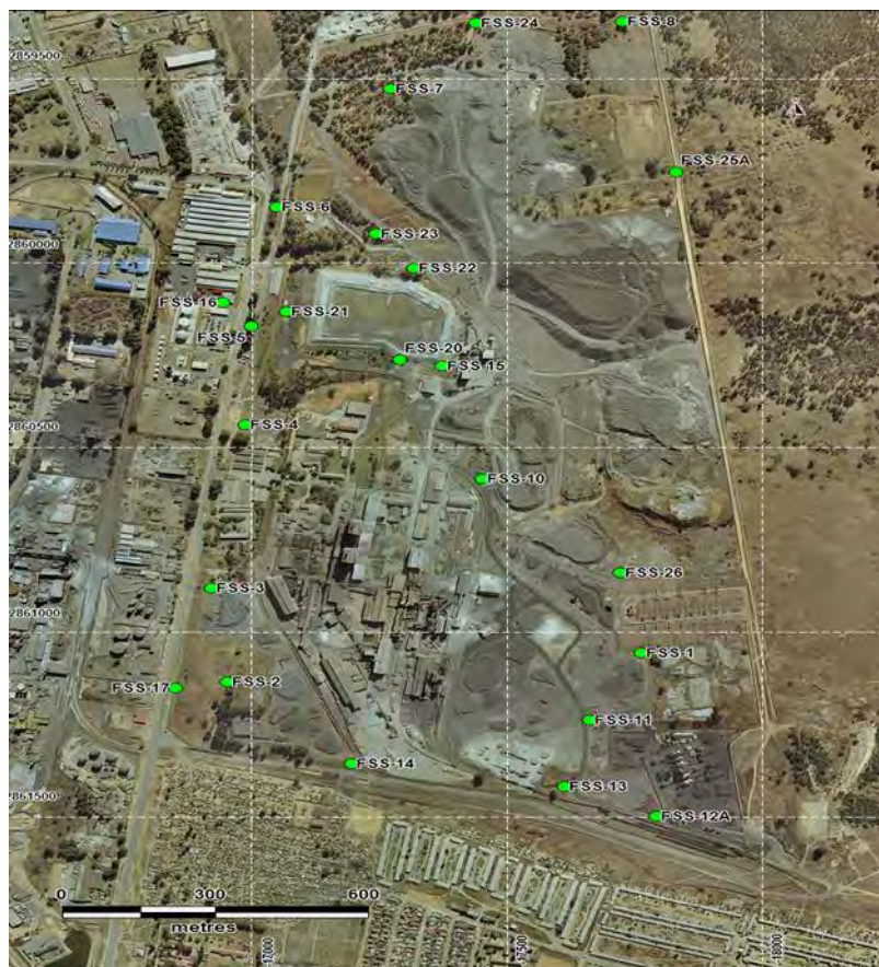
Figure 4.6(b): Shallow Perched Aquifer Monitoring Borehole localities.
