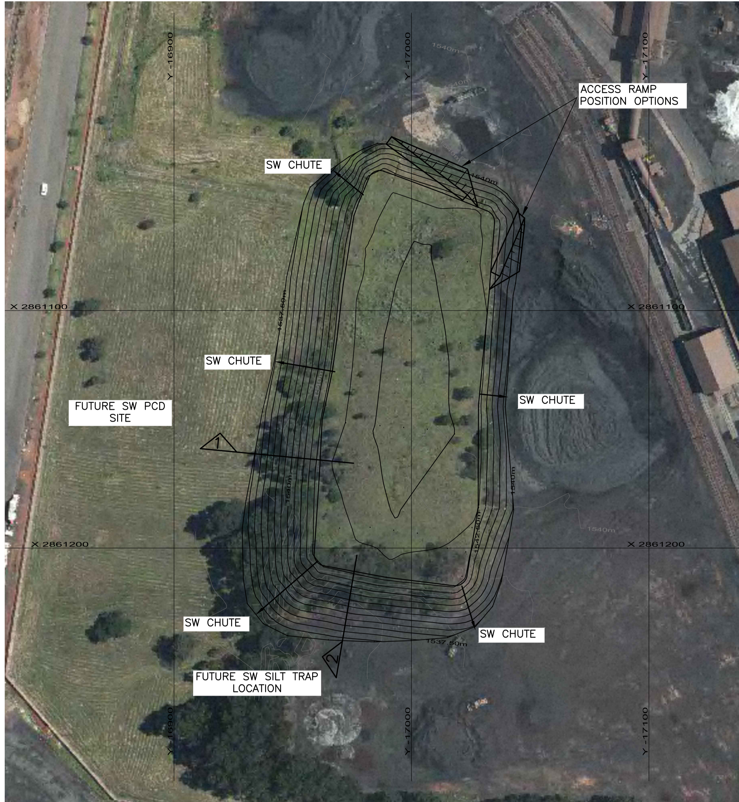
LAYOUT PLAN OF PROPOSED REHABILITATED SURFACE 1:1000
