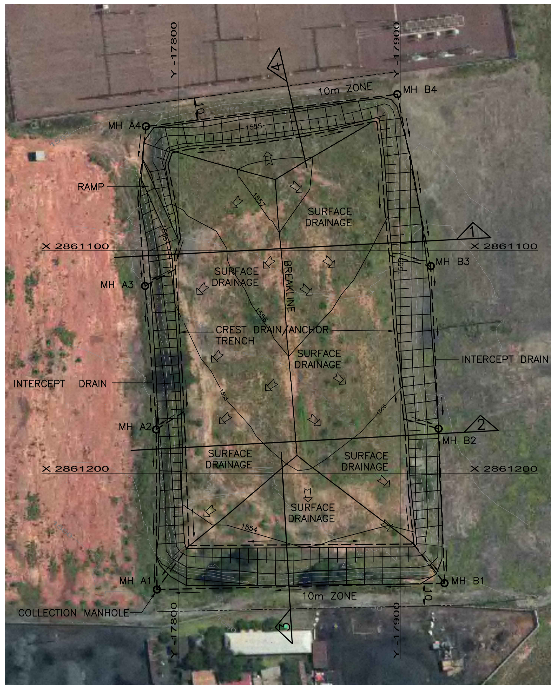
LAYOUT PLAN OF RE-PROFILED SURFACE 1:1000
