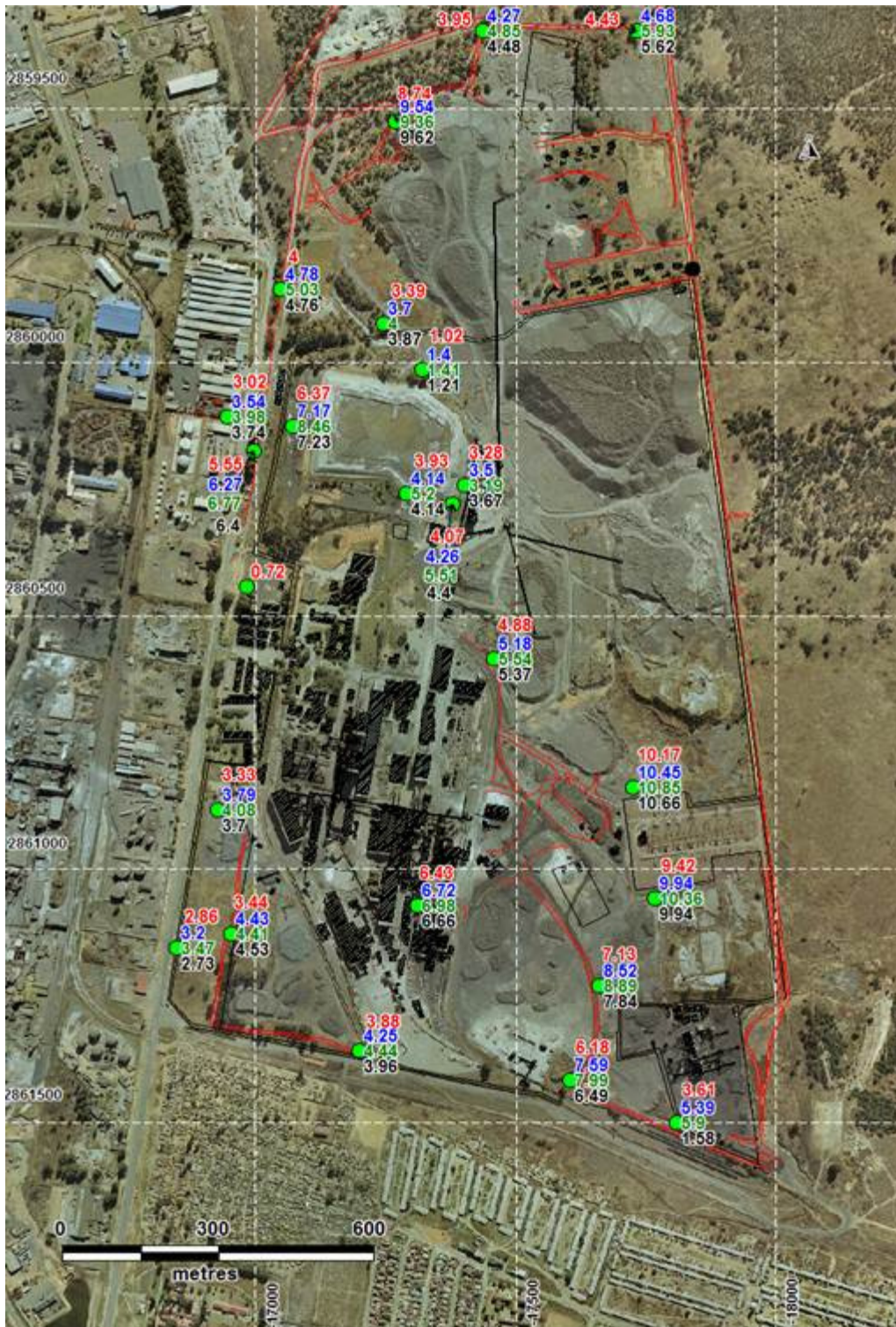
Figure 2.6: Ground water level data for 2012 – Deep Weathered monitoring boreholes. (Courtesy of JMA Consulting (Pty) Ltd)
