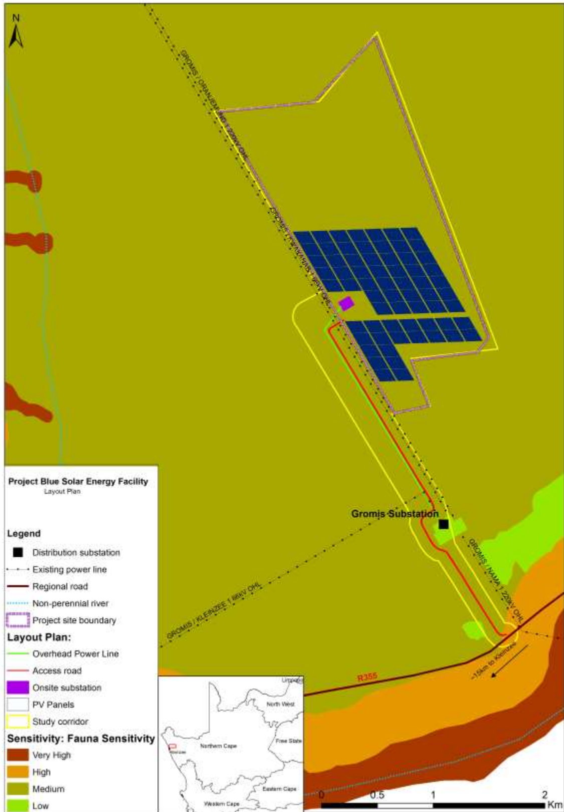
Figure 1: Environmental Sensitivity Map for the proposed Project Blue Solar Farm, north of Kleinsee, in the Northern Cape
