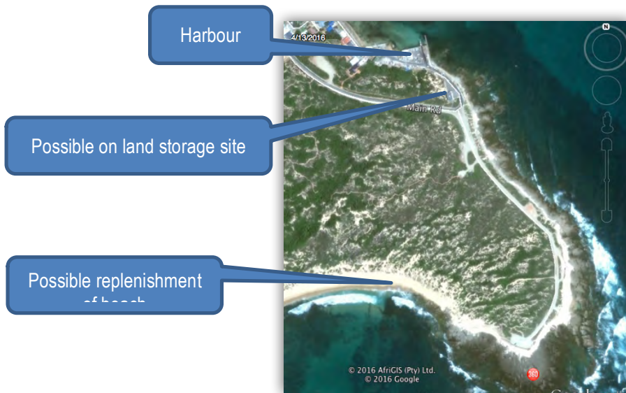
Figure 1.2.5.2: Proposed spoil areas for dredge material
