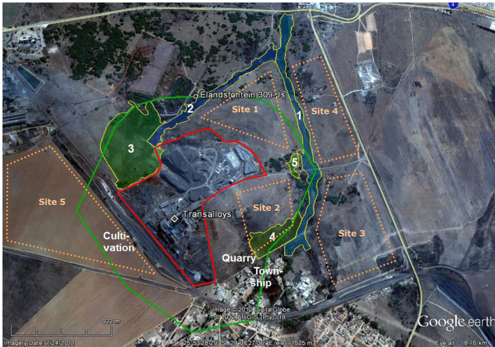
Figure 4.5: Wetlands (blue and green areas) delineated within 500m of the Transalloys industrial complex ( source: Ixhaphozi Environmental Services ) as mapped relative to the site alternatives 1 - 5
