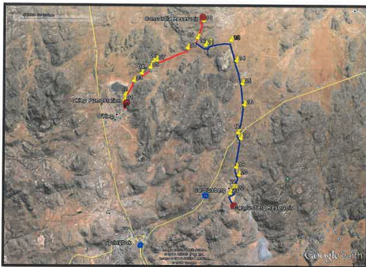
Figure 4: Google image showing the Concordia pipeline (Red) and the preferred Carolusberg route option (Blue)
