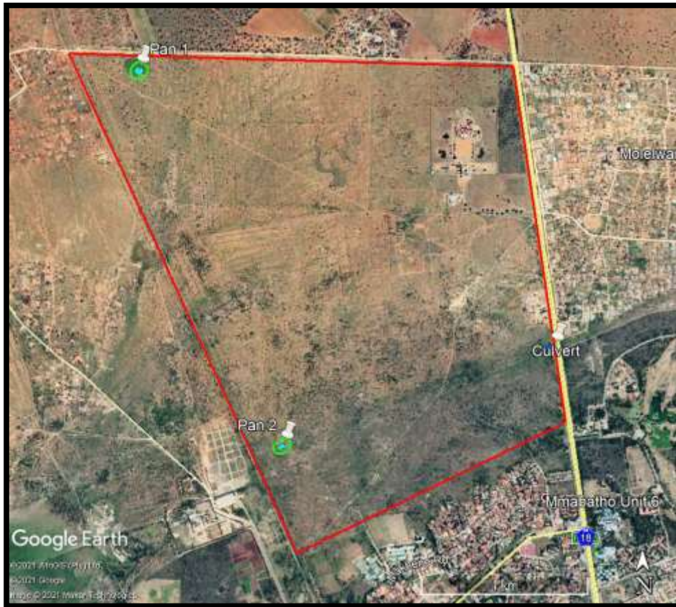
Figure 13: Indication of the small wetland depressions Pan 1 and Pan 2, as well as their buffer zones (32 m) at the site.
