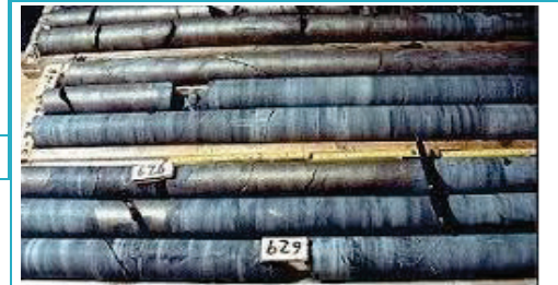
Rock core recovered for analysis
