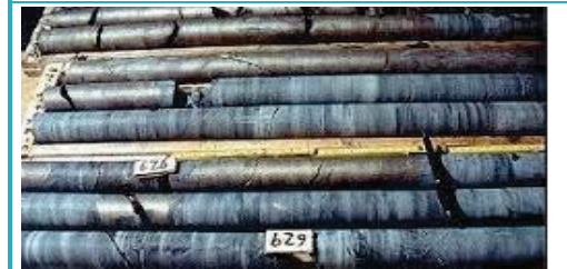
Rock core recovered for analysis
