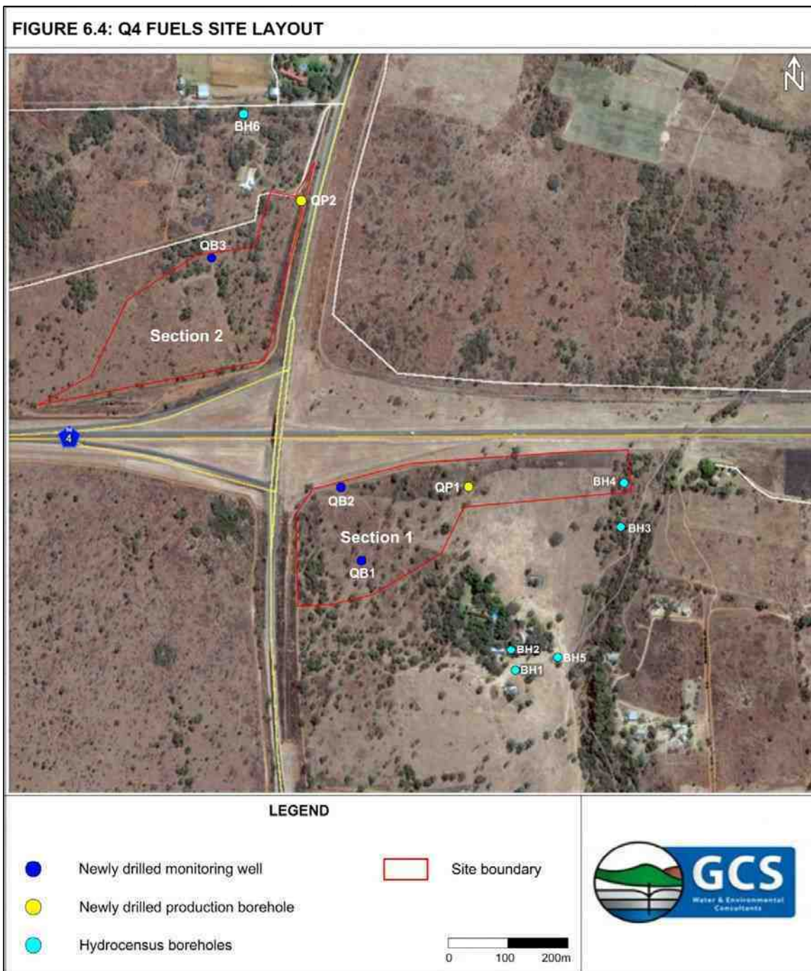
Figure 6-4: Site Layout and Hydrocensus Borehole Locality
