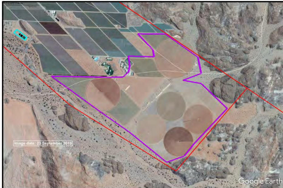
Figure 14. Aerial image (Google Earth™) of 29 September 2019, showing the main study area at Raap en Skraap (purple outline) with functioning centre-pivot irrigation. The one set of evaporations ponds is indicated by the light blue outline. The seasonal wash that flows from northeast to southwest was canalised.
