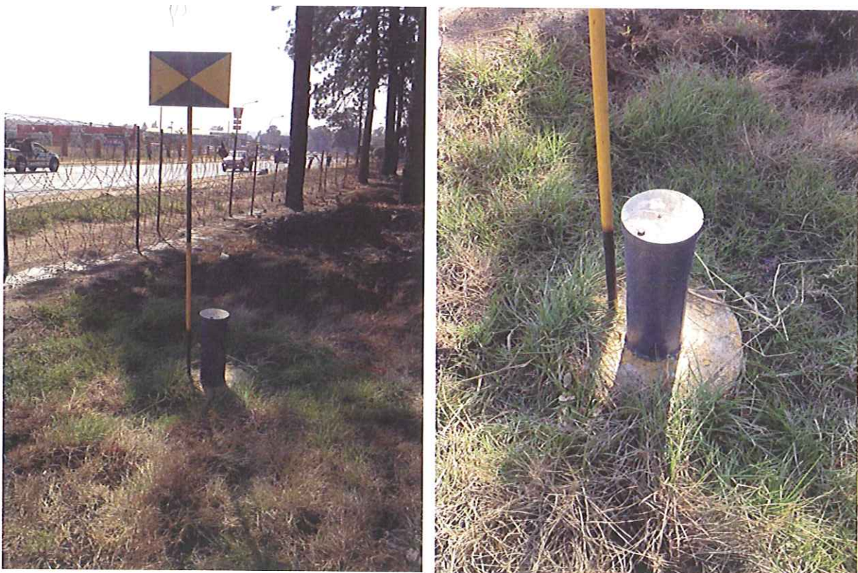
Plate 12-1: Example of a monitoring borehole
