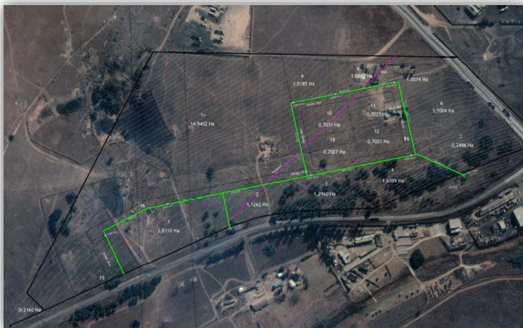
Figure 5: Stormwater Layout (SCIP Engineering Group, 2021)
