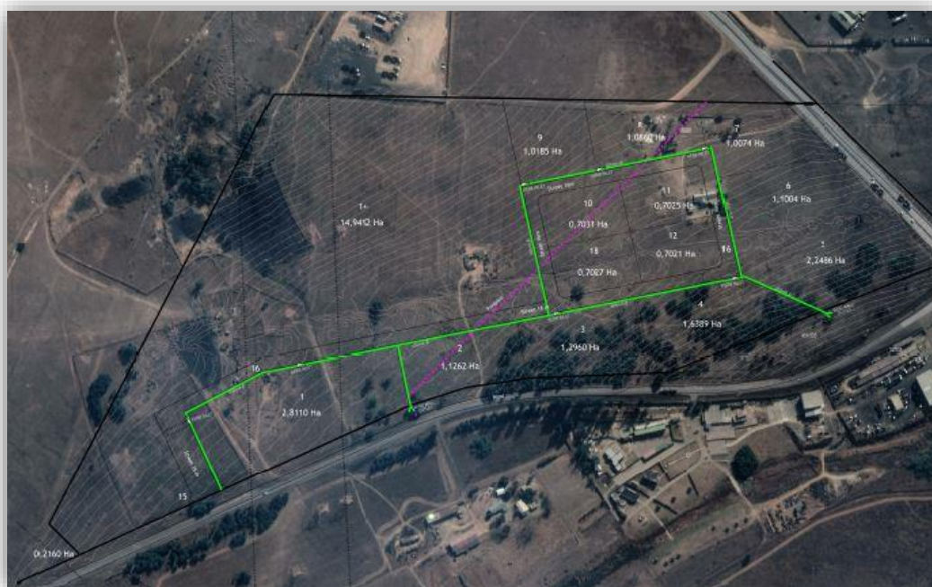
Figure 5: Stormwater Layout (SCIP Engineering Group, 2021)
