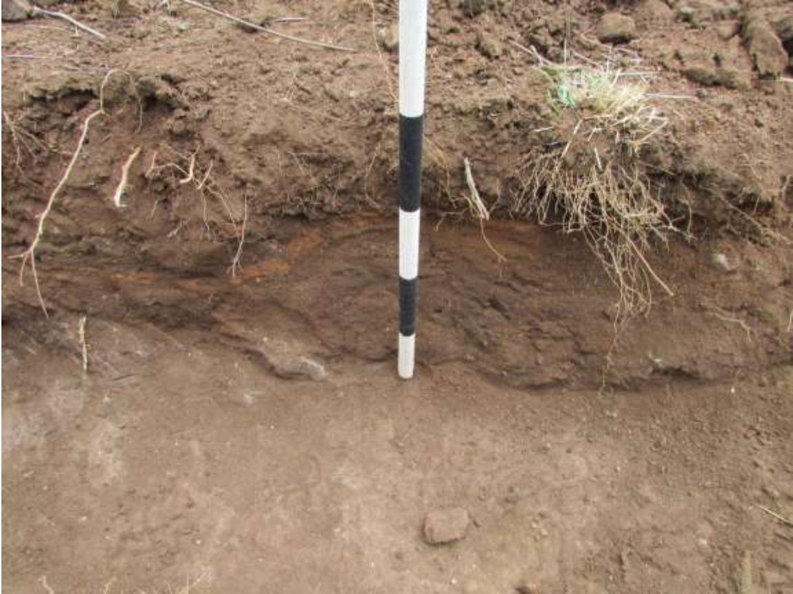
Figure 11: The stratigraphy in the 2 nd trench consists again of loose top soil overlaying a red, compacted layer of soil on top of an undisturbed hard dark-brown clay.
