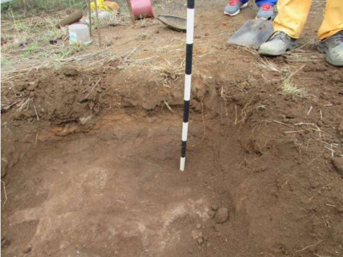
Figure 9: The stratigraphy in the trench consists of around 20cm of loose top soil overlaying a hard red layer of between 02cm & 05cm on top of a dark-brown compacted layer of clay.
