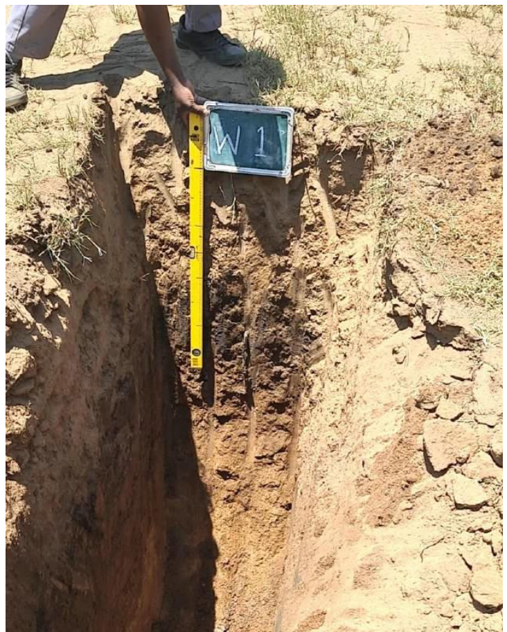
Photo 1. Typical soil profile (source: geotech Report)
