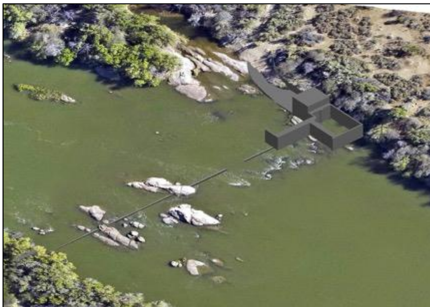
Figure 2: Conceptual diagram showing the proposed diversion weir and intake structure (from HydroSA (Pty) Ltd).
