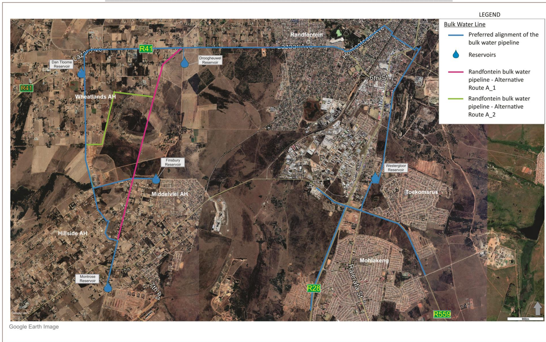
Figure 2_1: Locality Map of the Bulk Water Pipelines North of the N12 RAND WEST CITY LOCAL MUNICIPALITY - BULK INFRASTRUCTURE PROJECT
