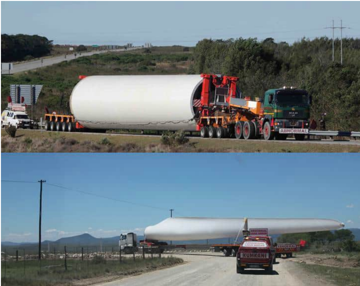
Figure 2-17: Tower section in low load configuration shown in top figure and blade shown in bottom figure
