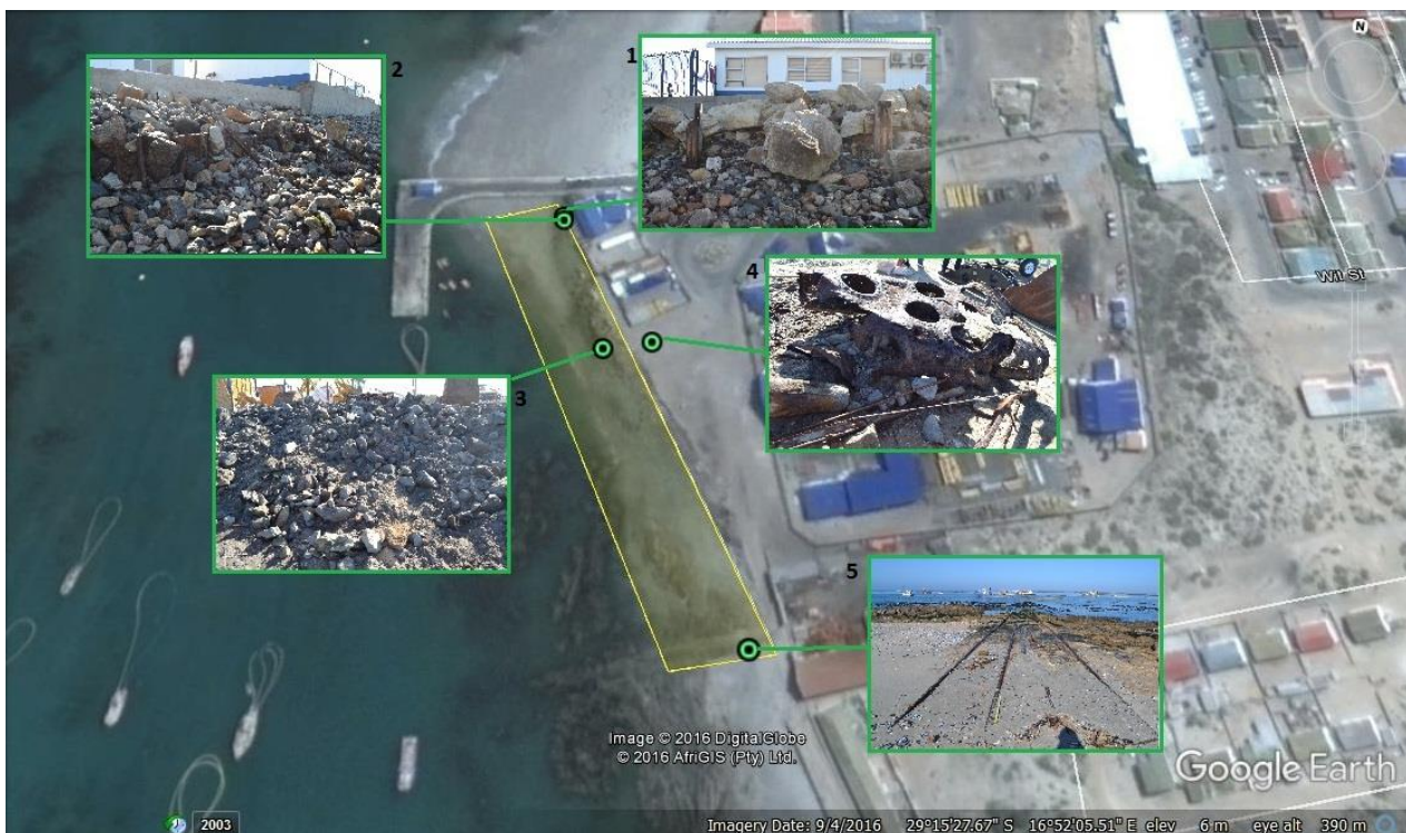
Figure 5: Polygon showing the area surveyed during the site assessment on the 14 th February 2017. Image 1: Remains of wooden jetty; Image 2: Old railway rails used to stabilise rock; Image 3: Rock covering area where the boiler was excavated; Image 4: Boiler and metal stockpile & Image 5: 19 th century slipway. (Source: Google Earth Imagery 9/04/2016).
