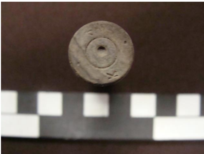
Figure 7: Headstamp of the .303 bullet casing.
