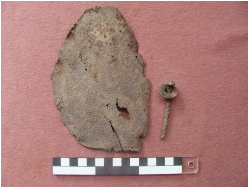
Figure 19 Piece of tin and a typical screw and washer used for fitting corrugated iron sheets.
