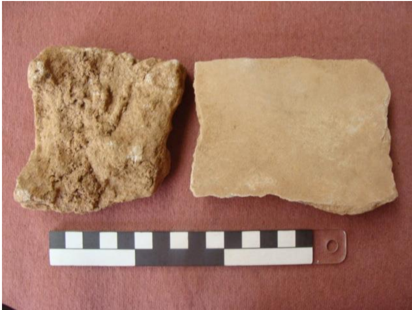
Figure 9 Pieces of concrete from Excavation 1. The smooth surface indicates that it most like is from a floor and therefore that the buildings here had a concrete floor.
