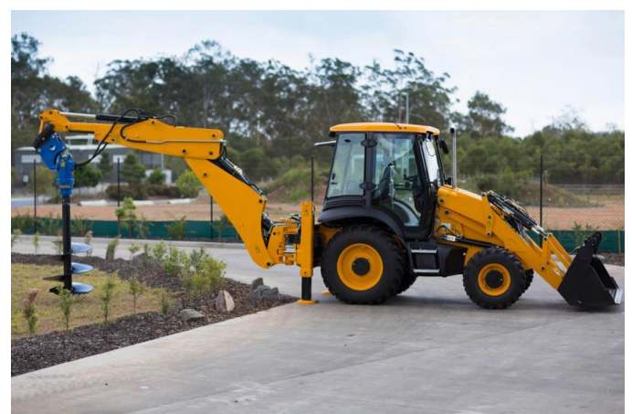
Plate 1: Example of a TLB mounted auger drill (Source: http://augerorqueusa.com )
