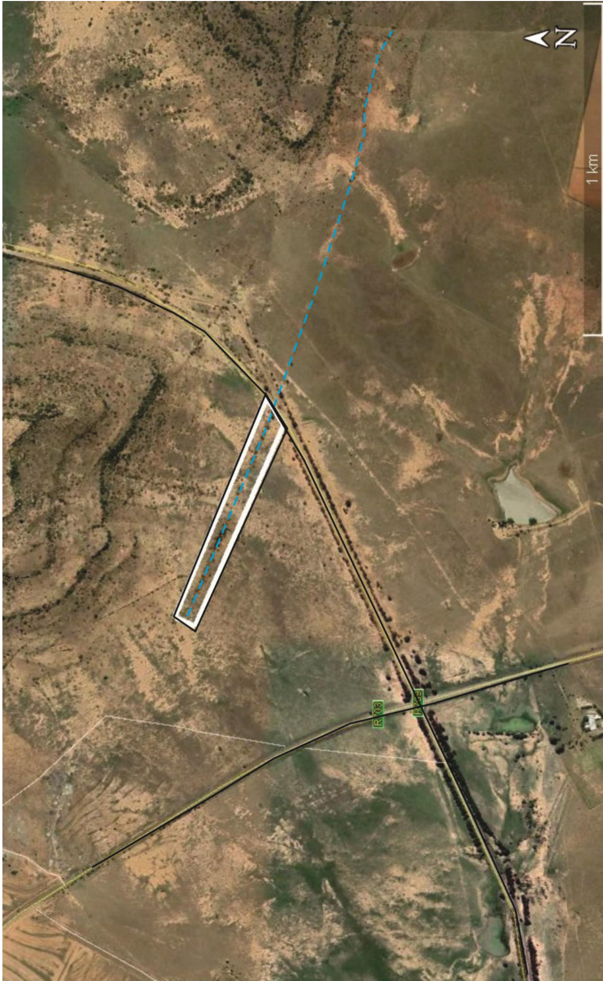
Figure 6. Aerial view of doolerite dyke (stippled line) traced out during survey.
